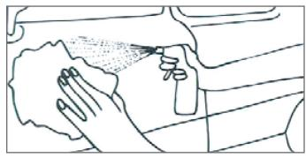
As every surface is dirty / dusty, it should be cleaned with petrol before start gluing.
