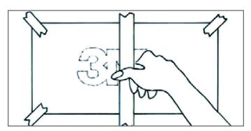
Align the adhesive tape (hinge) in the middle over the entire width.
