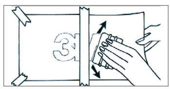
For gluing down 1 side of the foil, fold back the other half, avoiding any contact to the surface and keep it flat and straight. Starting at the hinge from the centre, press down the film and start scraping over the foil using the plastic blade.
