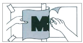
Fold back half of the foil, put the carrier flat up to the hinge and pull it off. Cut the carrier foil with a clean cut, using sharp knife or scissor, along the hinge.
