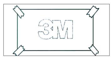
Place the lettering (label) on the desired position and align it with adhesive tape.
